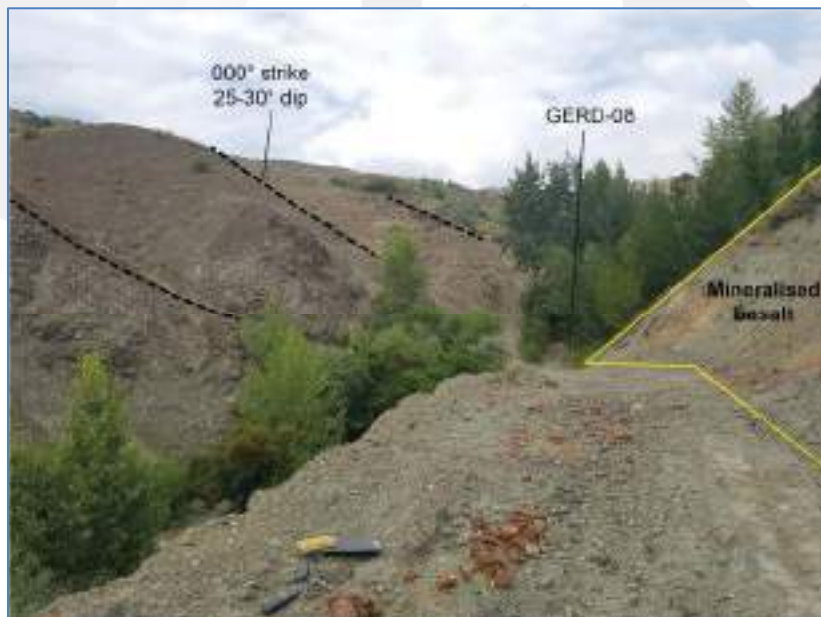
Figure 11: Area A. Looking north toward GERD-08. Photo indicating orientation of individual lava flows and outcropping mineralisation. Note: GERD-08 refers to the location of a drillhole collar.
