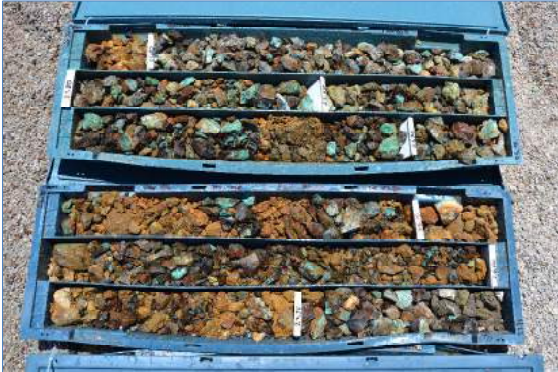
Figure 14: Area B, GERD-54 20.7 m to 27.8 m with abundant oxide Cu mineralisation.
